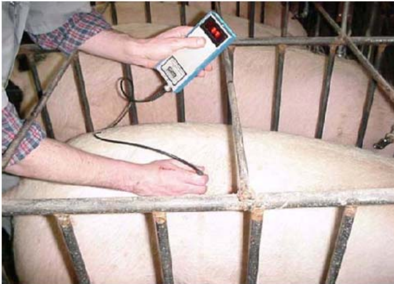
Figure 5. Illustration of Renco Lean Meater being used to measure backfat thickness
